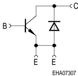
**Transistor Schematic Diagram**
